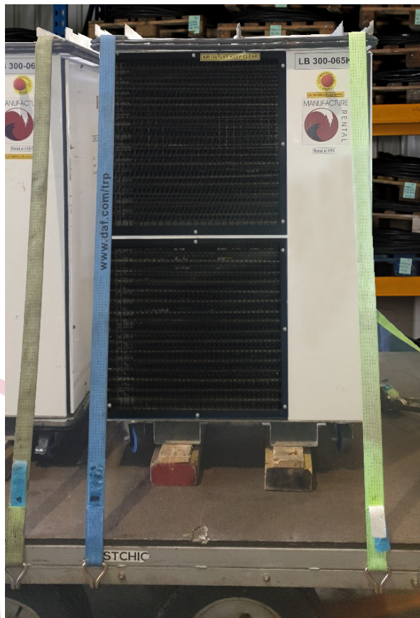
Figure 7- Strapping down castor mounted loadbank
