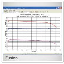
Equips DC load banks for performing constant-current or constant-power discharge tests, coupled with monitoring, data capture and reporting. Again, control is available for multiple load banks via PC/HHT100.
