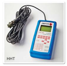
The HHT100 hand held field controller is suitable for all micro-processor controlled load banks, providing portable, robust control up to100m, with basic instrumentation, pre-set load programmes and M-start facility.
